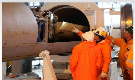
Pig launch tray removal launcher
